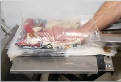
Ergonomic loading guides ease product loading
